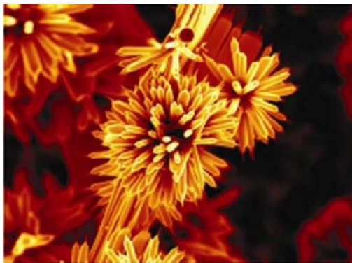
Figure 18. Zinc oxide nanostructures synthesized by a vapor-solid process. (Image courtesy of Prof. Zhong Win Lang of Georgia Tech.)
